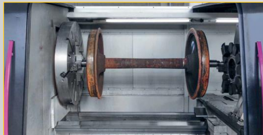
LATHE FOR RAILWAY AXLES
